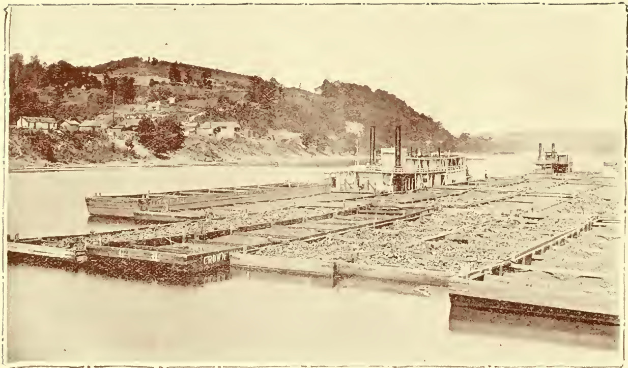
View on the Great Kanawha River. A fleet of loaded coal barges (with two tow boats,) tied up in the No. 6 or Charleston Pool. A coal barge is generally 25 feet wide, 130 feet long, draught from 6 to 7 feet. Capacity loaded to 6½ feet is about 14,000 bushels or 560 tons.
